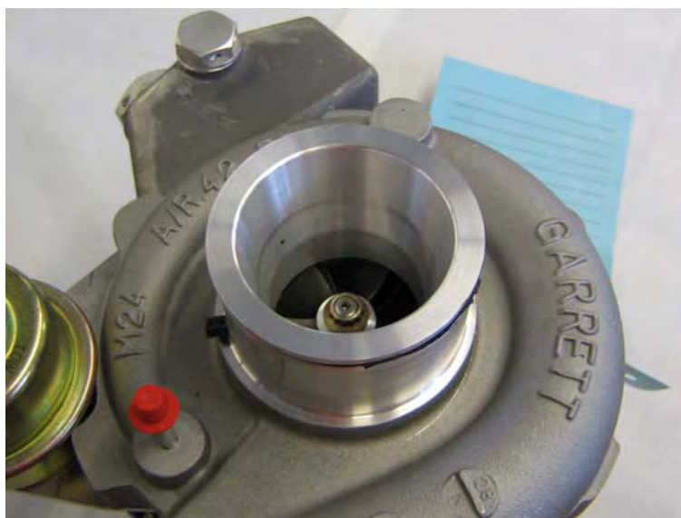
Fig. 6.46 Air restrictor of the turbocharger (2)
