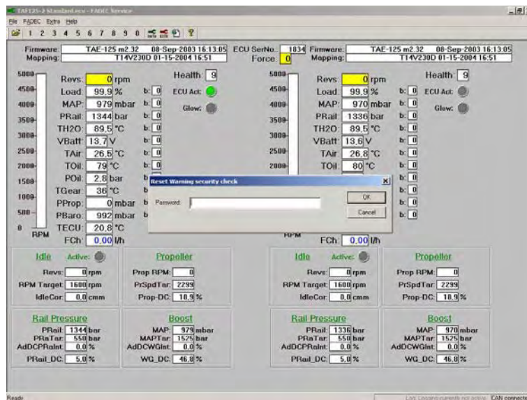
Fig. 6.31 FADEC read-out - Enter password
