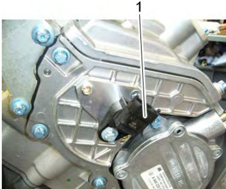
Fig. 6.7 Camshaft sensor 2 1 Camshaft sensor 2 FADEC B (2 of 2)
