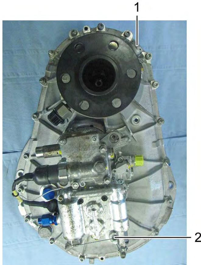
Fig. 6.26 Gearbox oil filler screw and inspection glass
