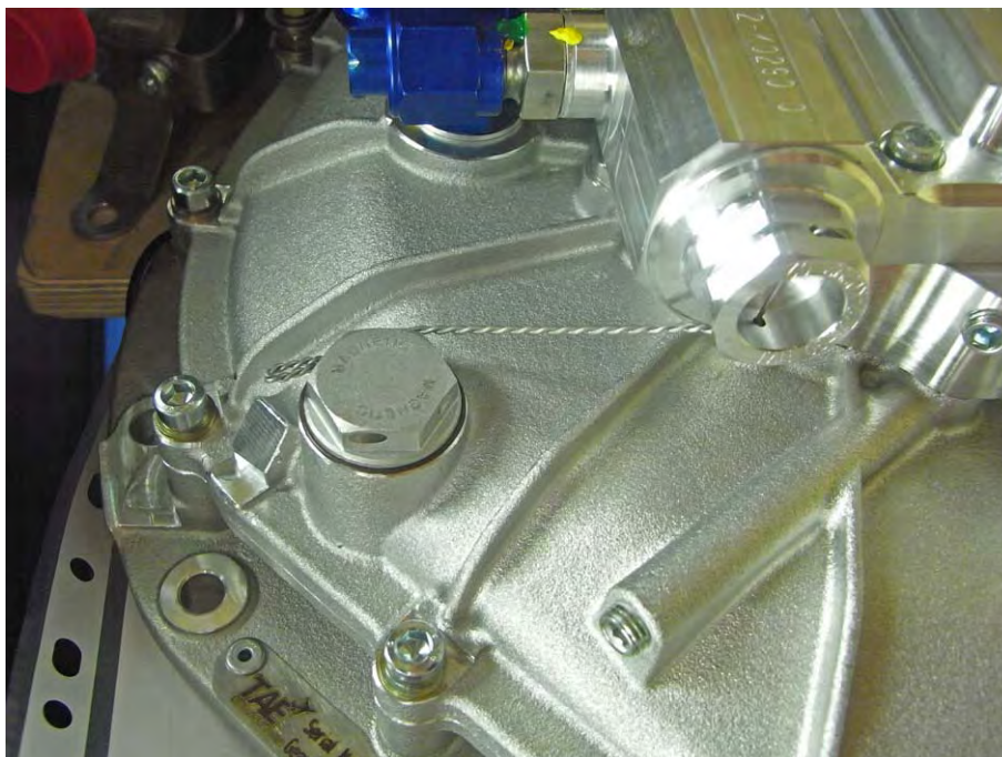
Fig. 6.16 Lock wiring between oil drain plug and oil filter cap
