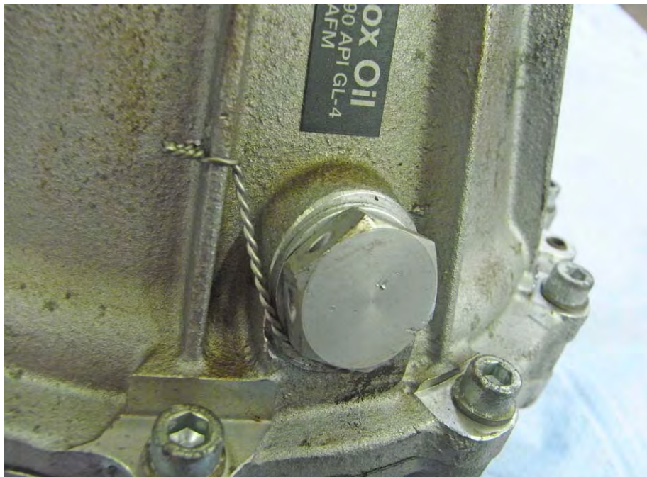
Fig. 6.48 Lock wiring the oil filler screw
