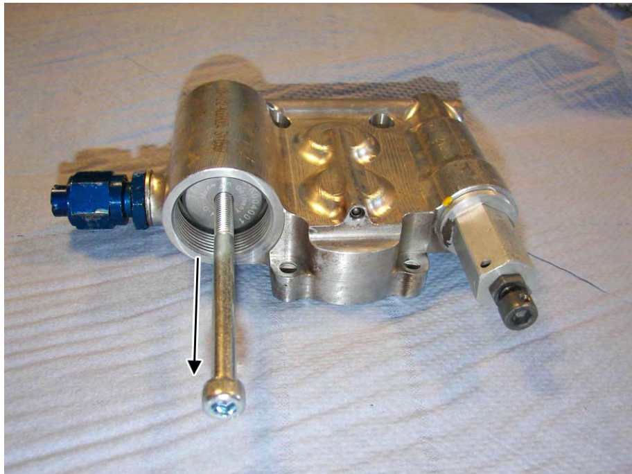
Fig. 6.18 Removal of gearbox oil filter
