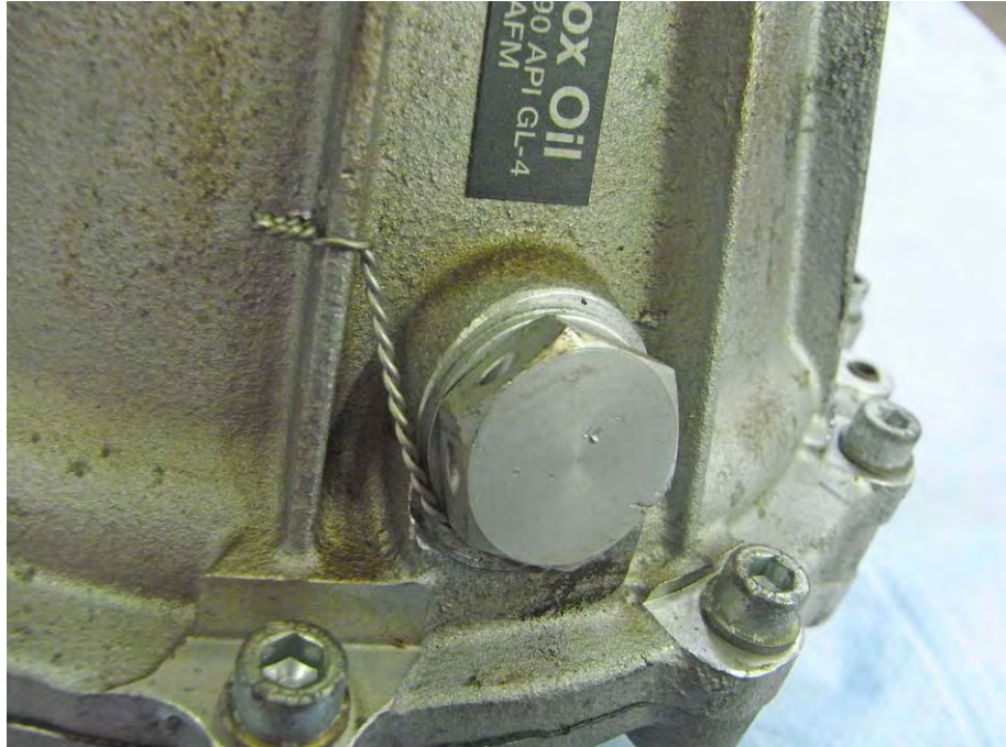
Fig. 6.55 Lock wiring the oil filler screw
