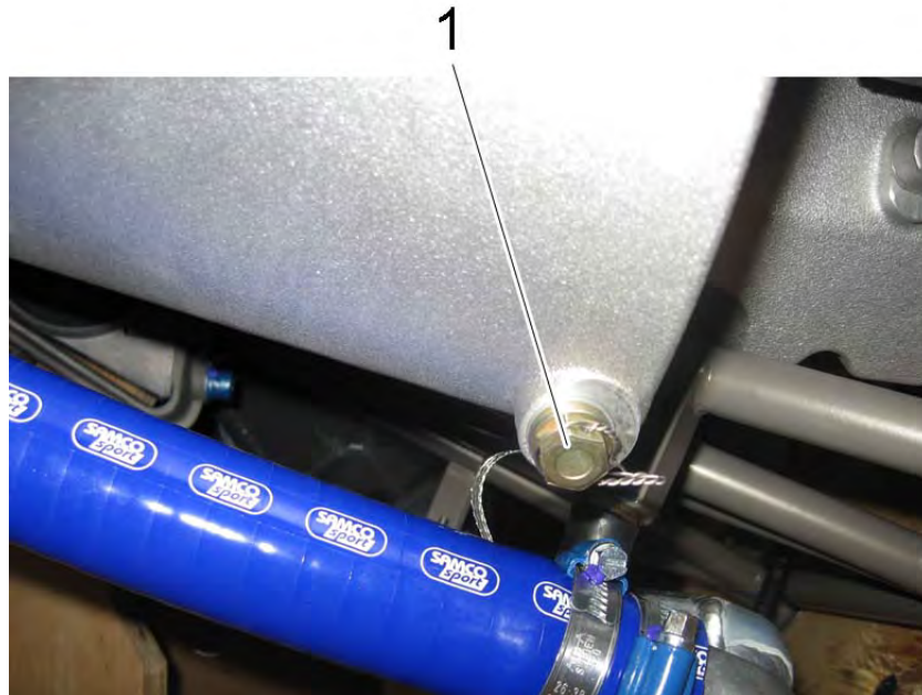
Fig. 6.1 Oil drain plug
