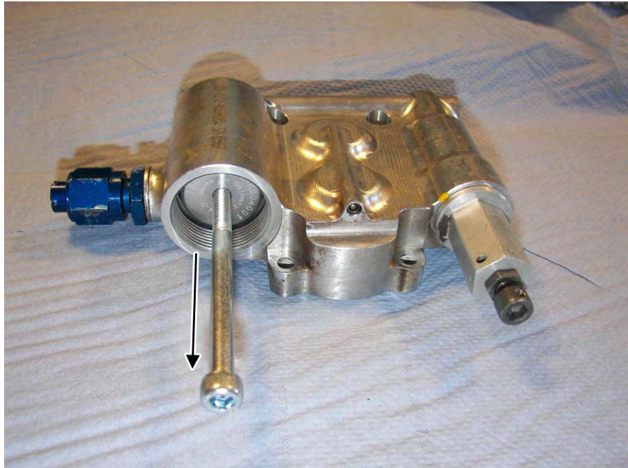
Fig. 6.50 Removal of gearbox oil filter
