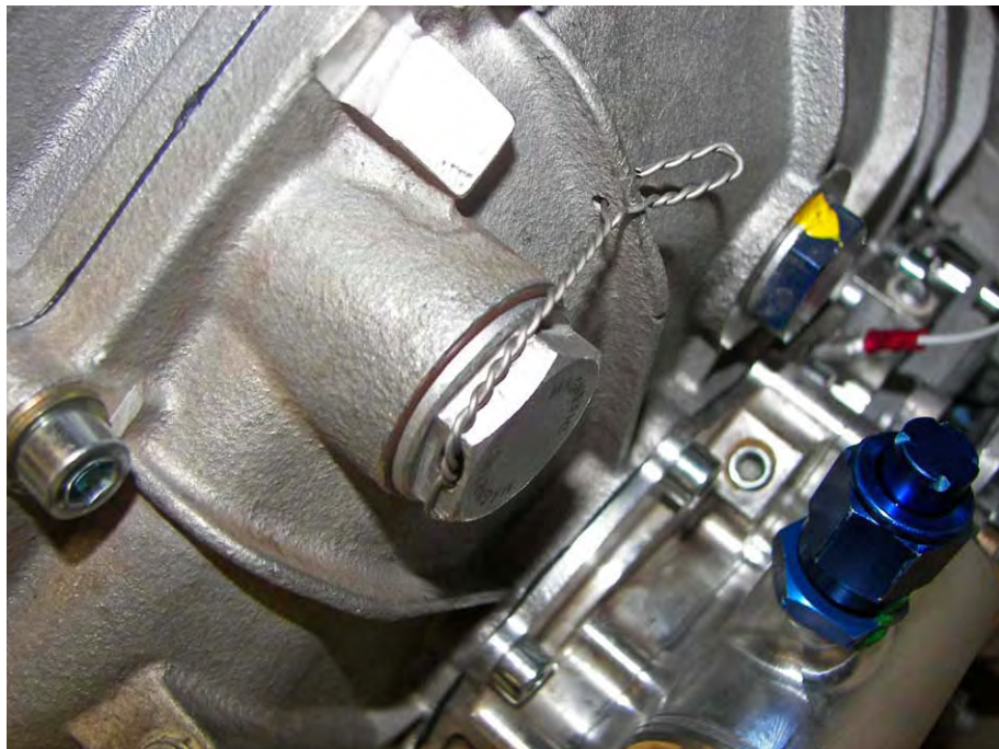
Fig. 6.54 Lock wiring the oil drain screw
