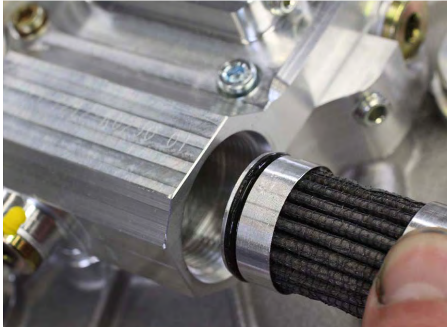
Fig. 6.14 Mounting direction of the oil filter
