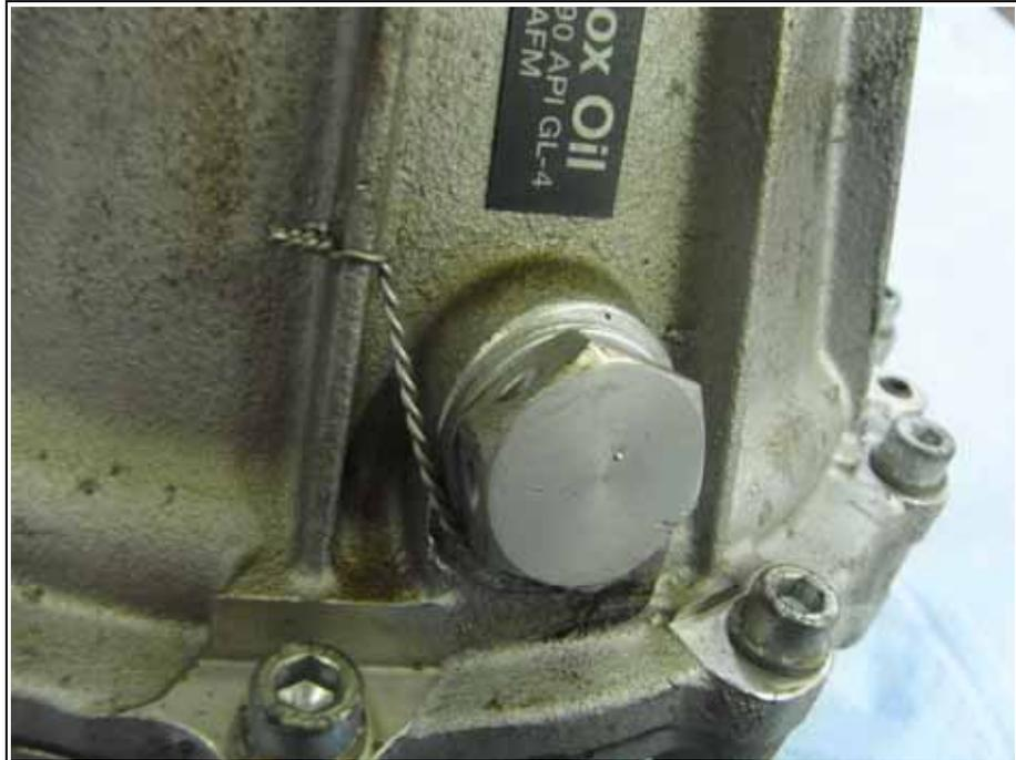
Fig. 6.55 Lock wiring the oil filler screw
