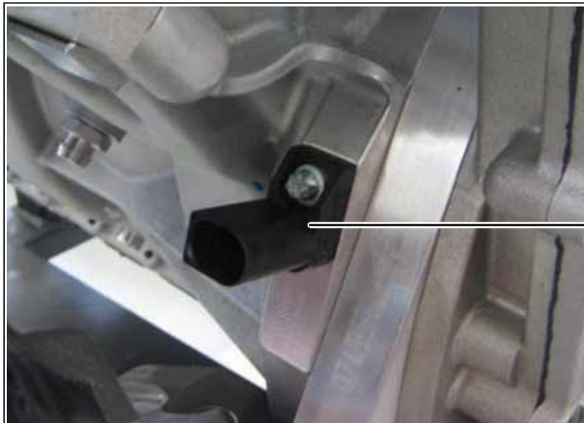
Fig. 6.8 Crankshaft sensor 1
