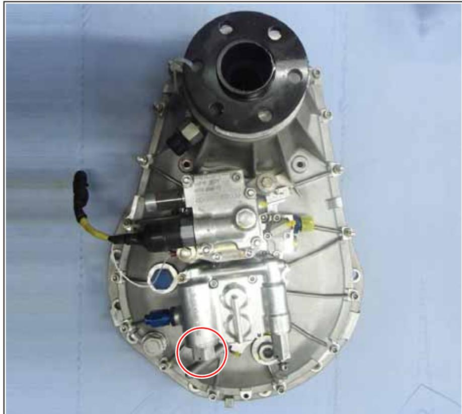
Fig. 6.16 Position of the oil filter cap
