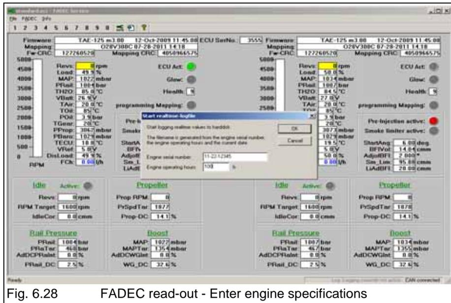
Fig. 6.28 FADEC read-out - Enter engine specifications
