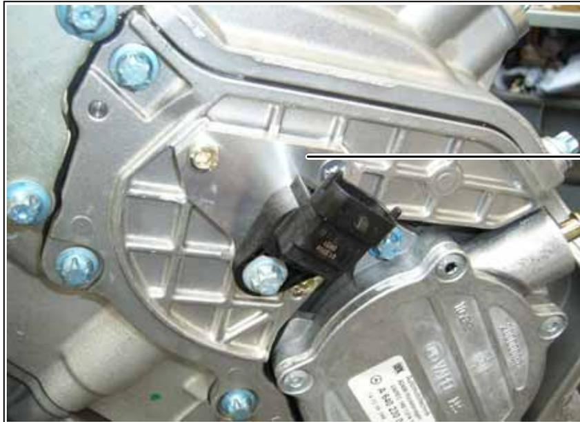
Fig. 6.7 Camshaft sensor 2
