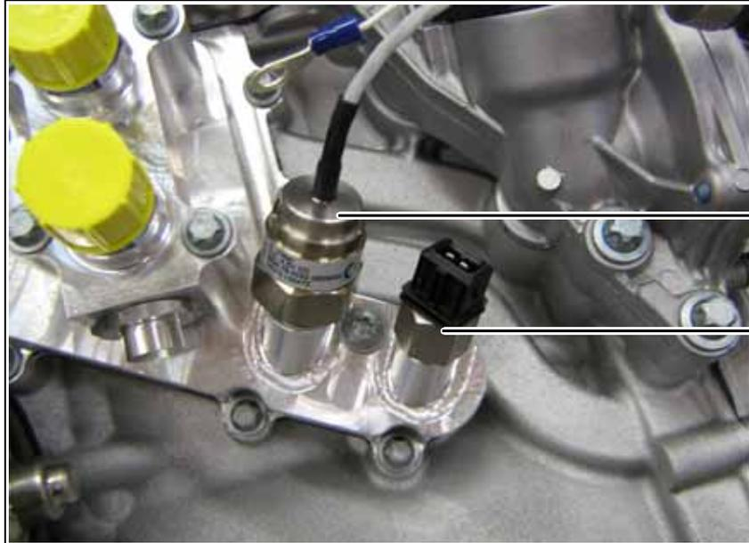
Fig. 6.11 Oil pressure- and oil temperature sensor
