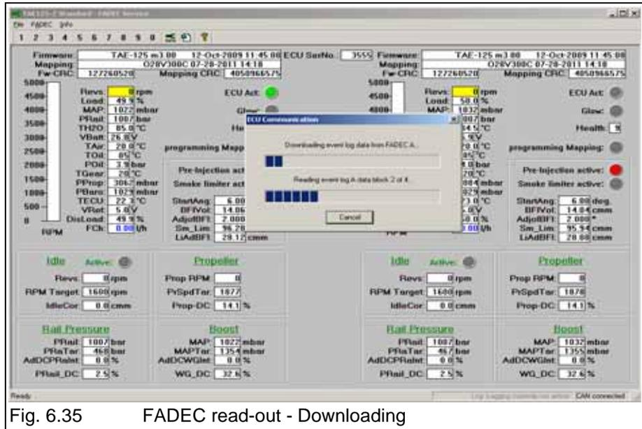
Fig. 6.35 FADEC read-out - Downloading
