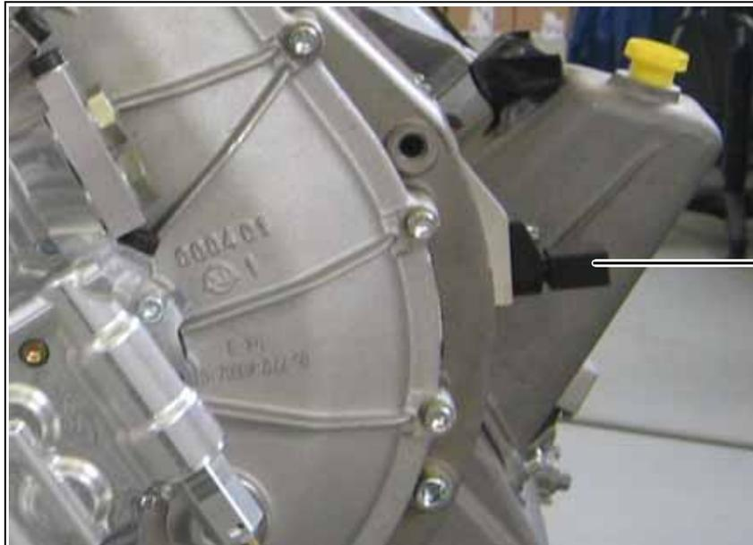
Fig. 6.9 Crankshaft sensor 2
