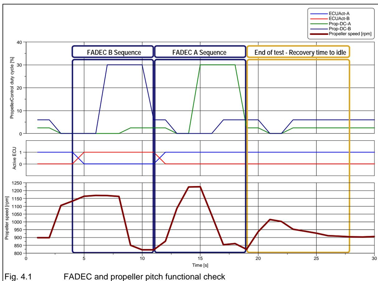
Fig. 4.1 FADEC and propeller pitch functional check
