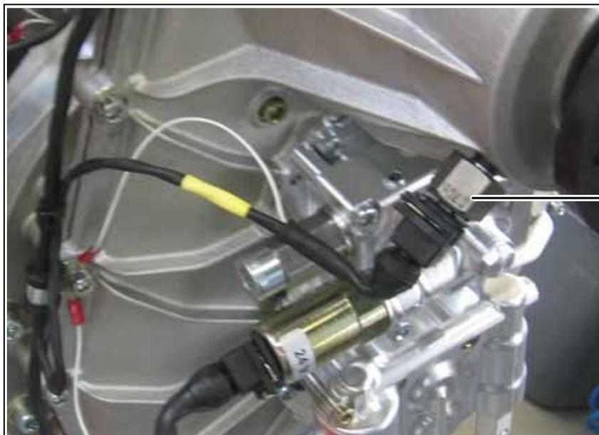
Fig. 6.10 Gearbox temperature sensor
