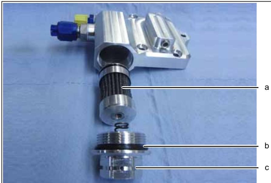
Fig. 6.14 Gearbox oil filter assembling
