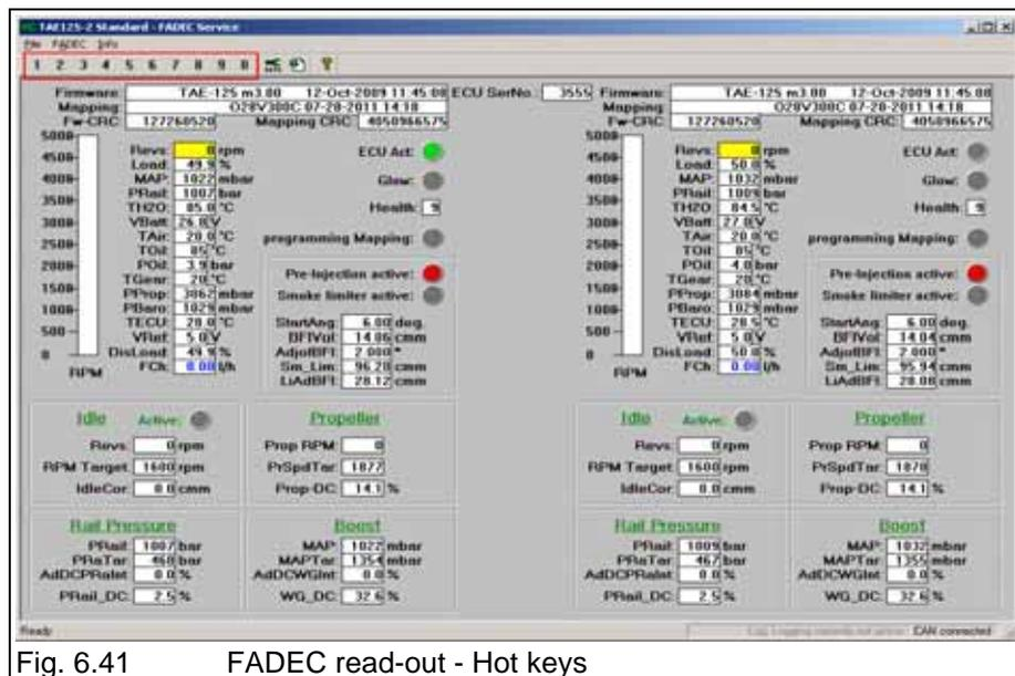
Fig. 6.41 FADEC read-out - Hot keys
