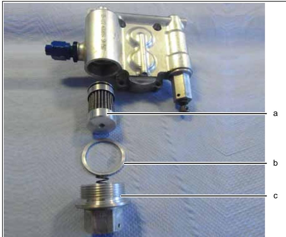
Fig. 6.18 Gearbox oil filter assembling
