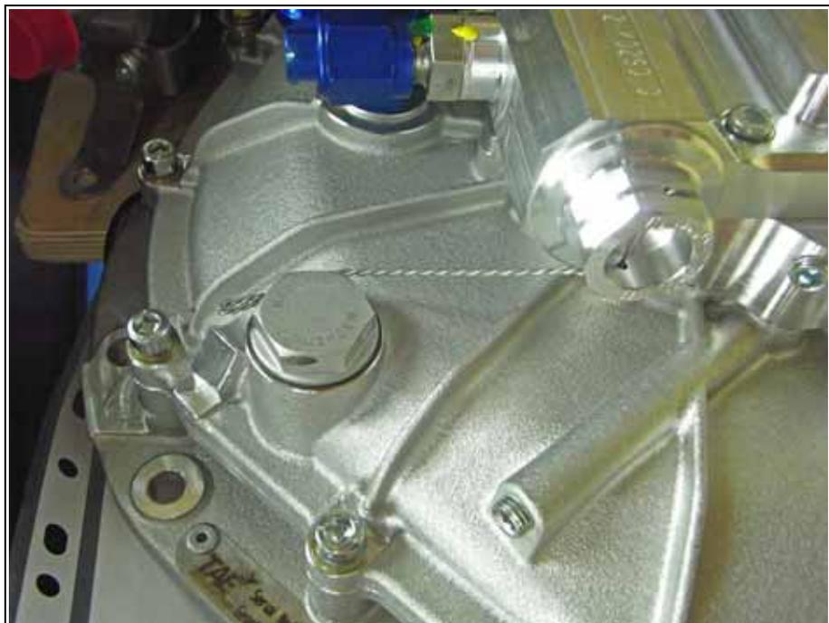
Fig. 6.15 Lock wiring between oil drain plug and oil filter cap
