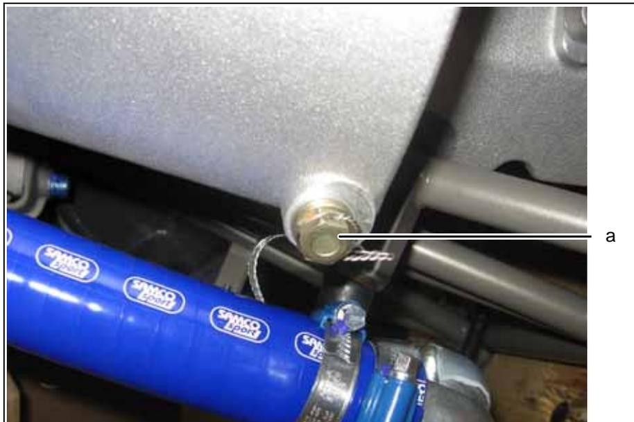
Fig. 6.1 Oil drain plug
