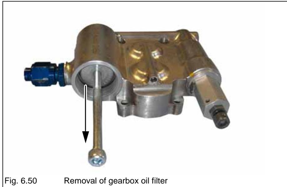
7. Insert the new gearbox oil filter. For mounting direction see Fig. 6.51 and Fig. 6.52.
