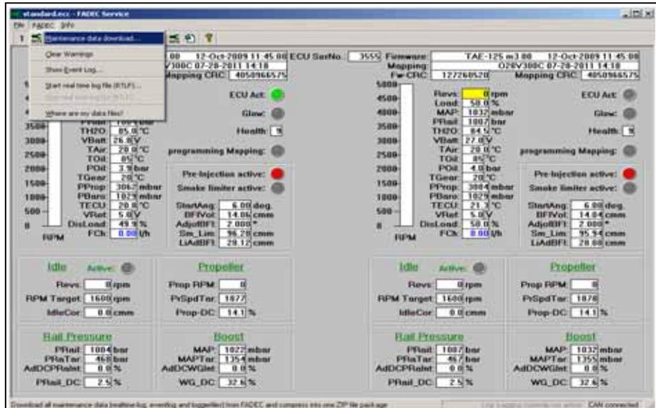
Fig. 6.32 FADEC read-out - Maintenance data download
