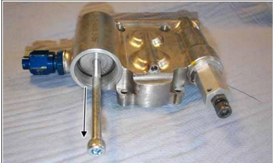
Fig. 6.17 Removal of gearbox oil filter
