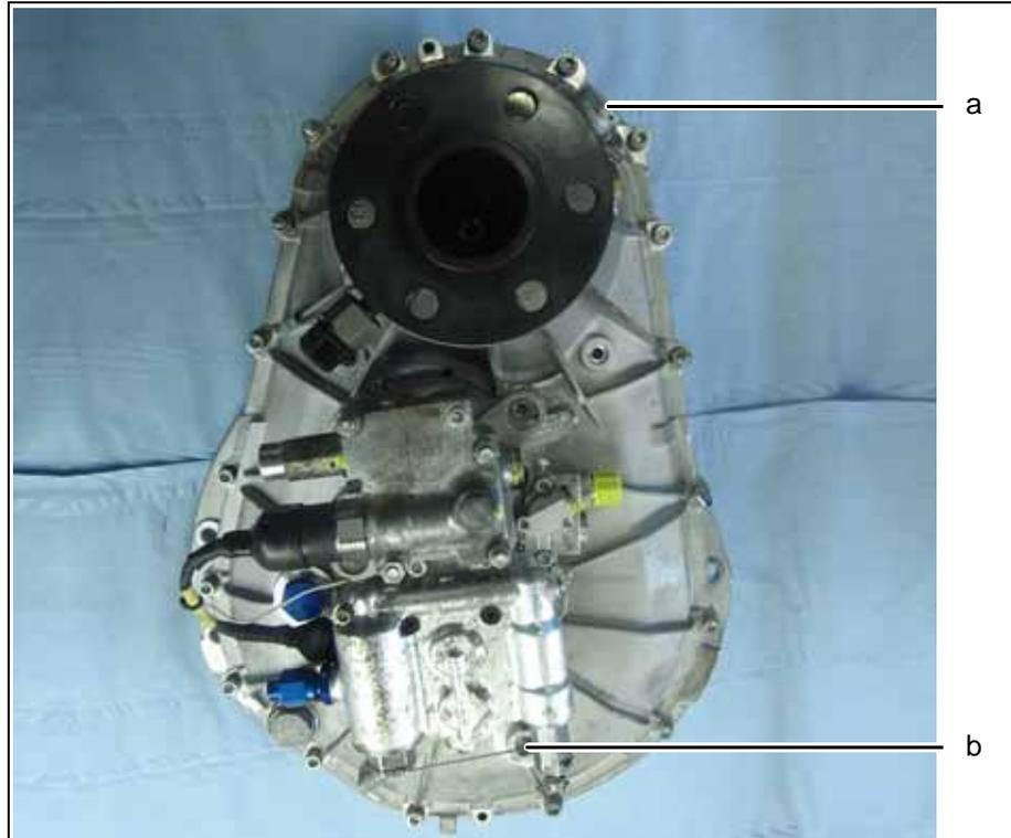
Fig. 6.25 Gearbox oil filler screw and inspection glass
