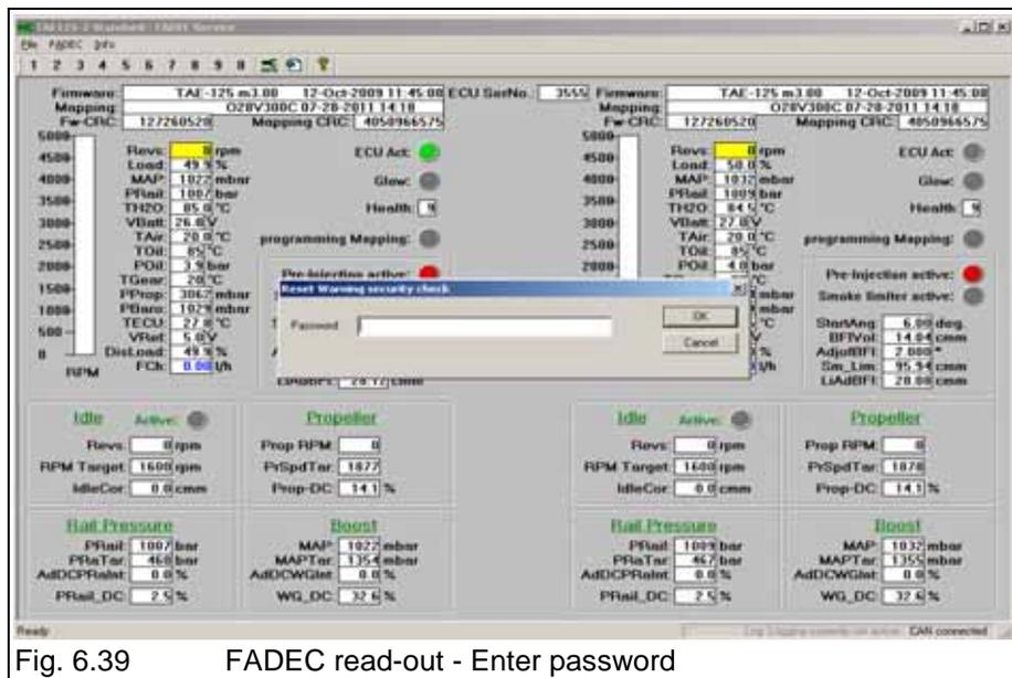
Fig. 6.39 FADEC read-out - Enter password
