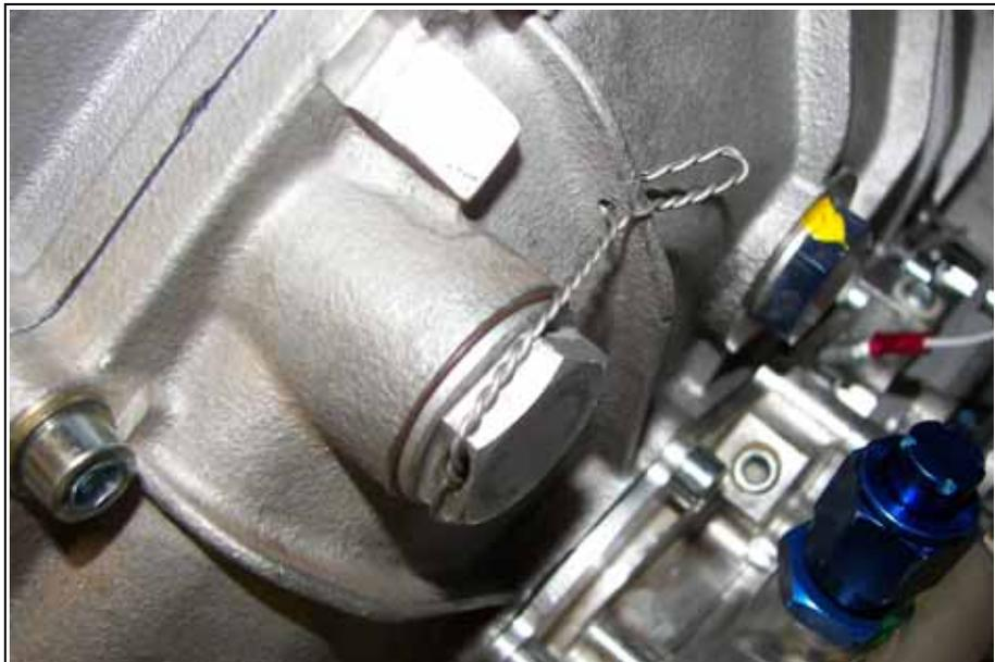
Fig. 6.54 Lock wiring the oil drain screw
