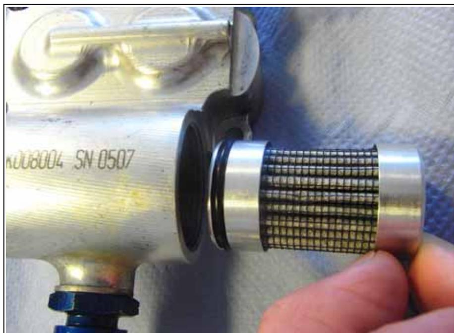
Fig. 6.19 Mounting direction of the oil filter
