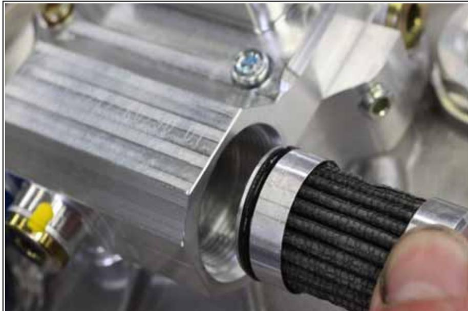
Fig. 6.13 Mounting direction of the oil filter
