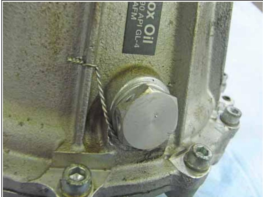
Fig. 6.26 Lock wiring the oil filler screw
