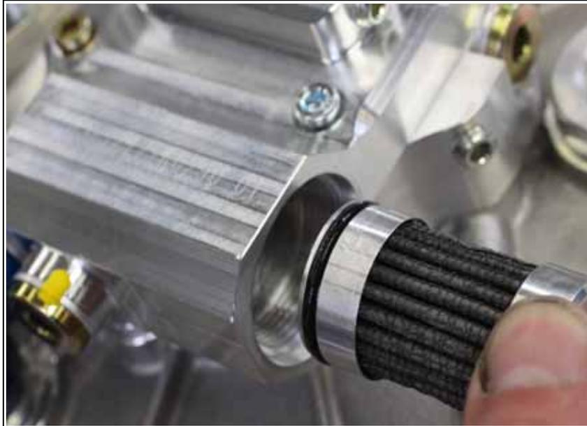
Fig. 6.45 Mounting direction of the oil filter
