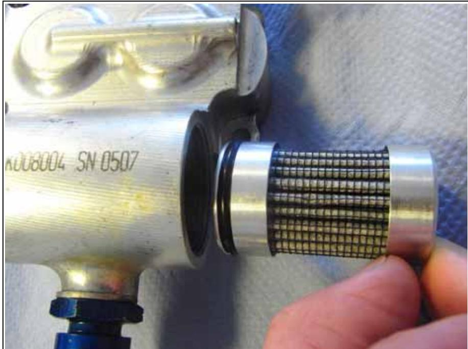
Fig. 6.52 Mounting direction of the oil filter
