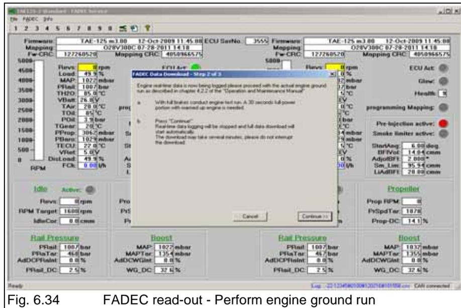
Fig. 6.34 FADEC read-out - Perform engine ground run
