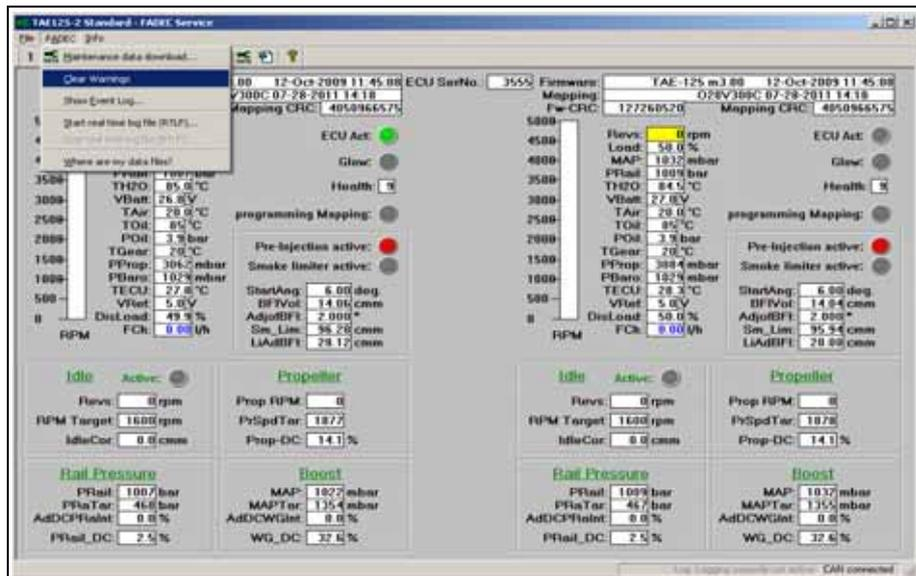
Fig. 6.38 FADEC read-out - Clear warnings
