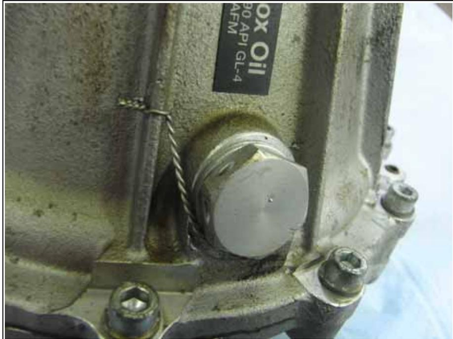
Fig. 6.48 Lock wiring the oil filler screw
