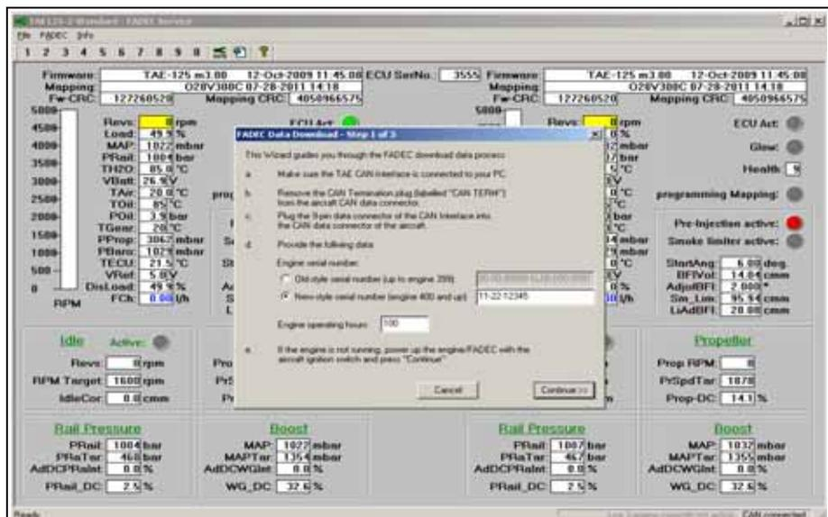
Fig. 6.33 FADEC read-out - Enter engine specifications
