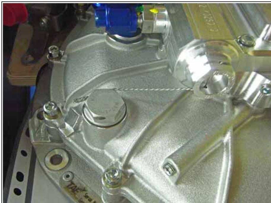
Fig. 6.47 Lock wire between the oil drain plug and the filter cap
