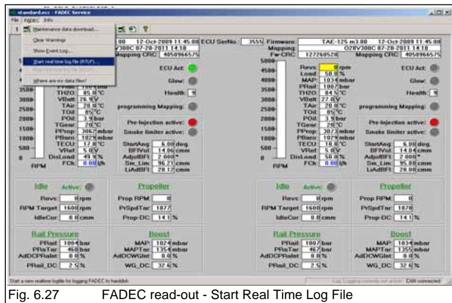
Fig. 6.27 FADEC read-out - Start Real Time Log File
