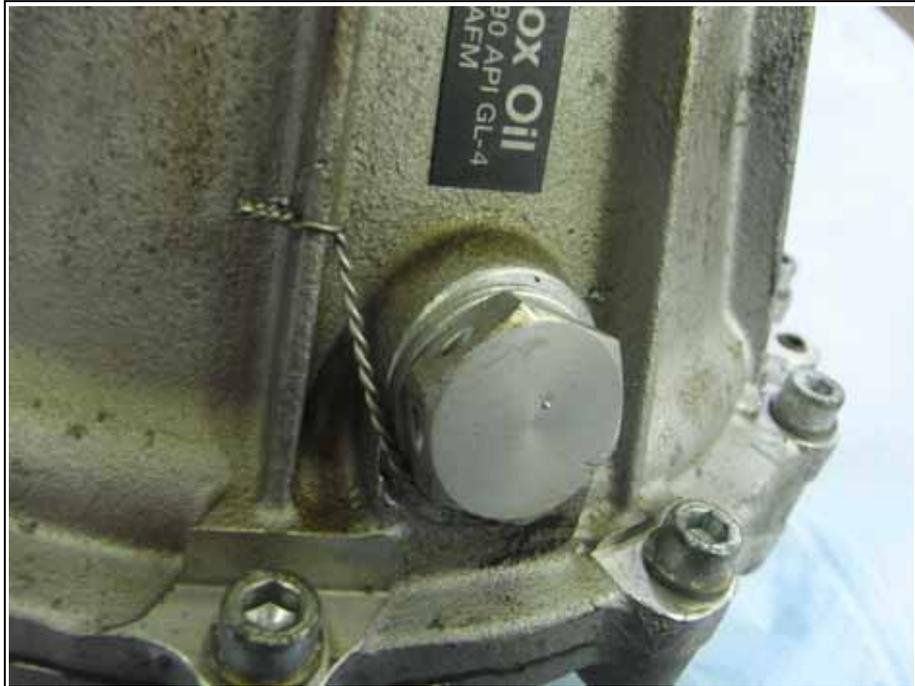
Fig. 6.23 Lock wiring the oil filler screw
