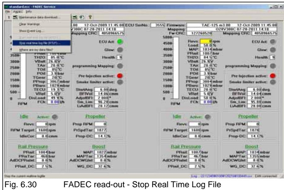
Fig. 6.30 FADEC read-out - Stop Real Time Log File
