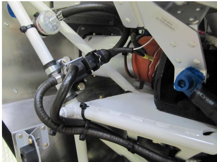
Abbildung 6 Neue Position des Waste-Gate-Ventils Figure 6 New position of waste gate valve
