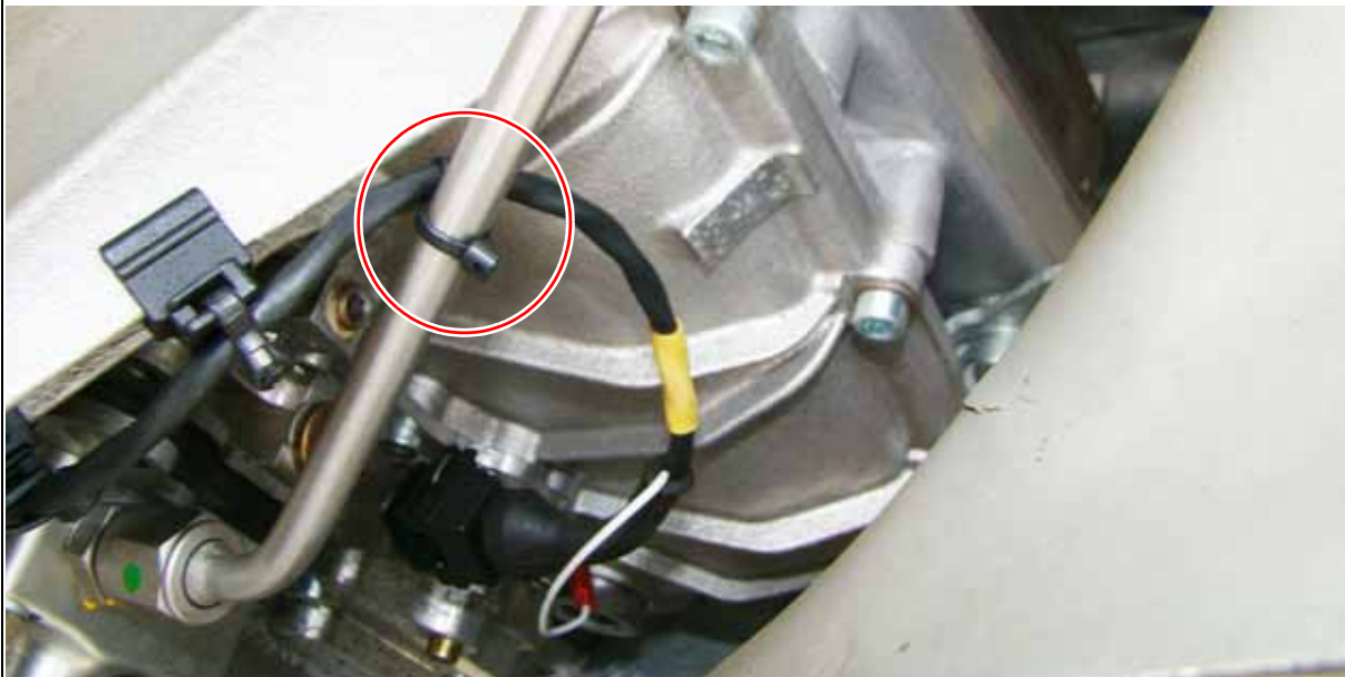
Figure 8 non-approved attachment: gearbox pipe
