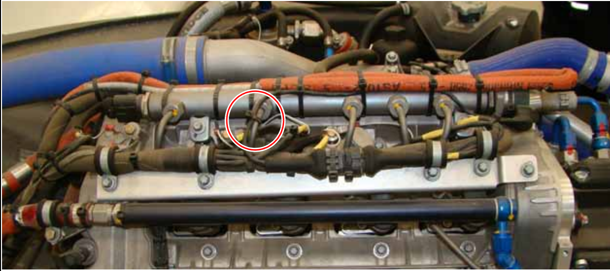
Figure 2 non-approved attachment: injector rail
