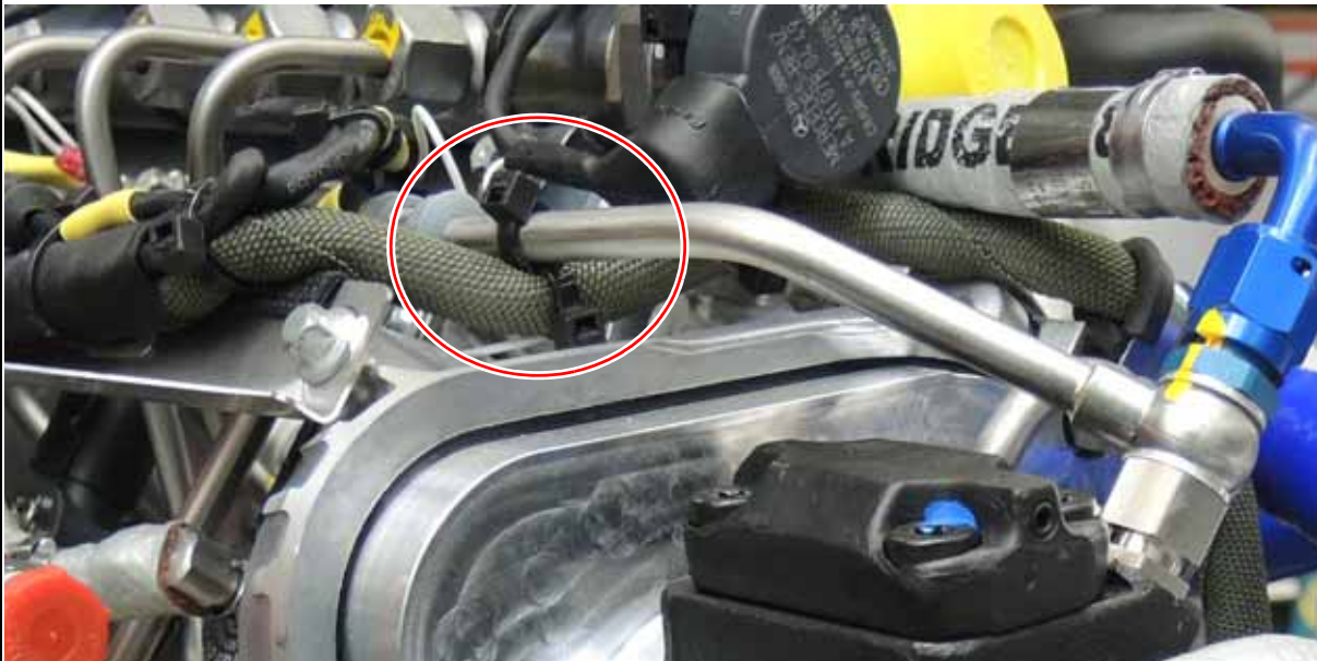
Figure 7 non-approved attachment: fuel return pipe
