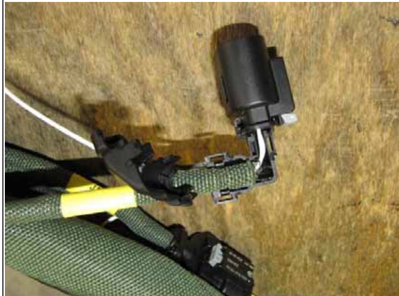
Figure 12 new alignment of the backshell
