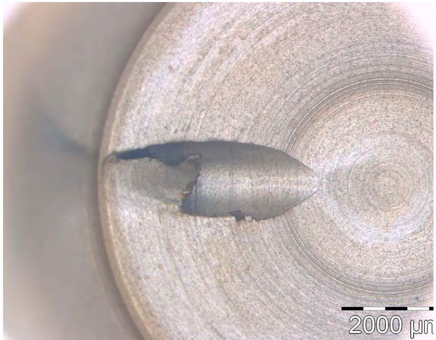
Figure 4 – Magnification of the chip inside of the oil filler plug
