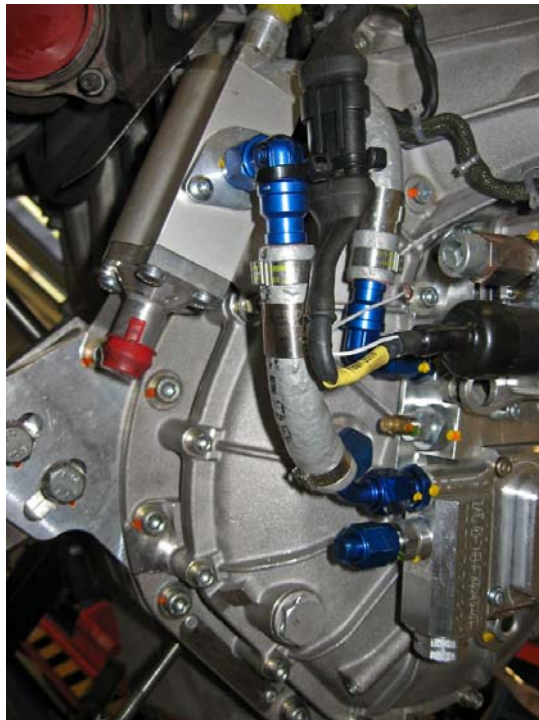
Bild 1 / Fig. 1 Old hose pump – gearbox oil cooler
