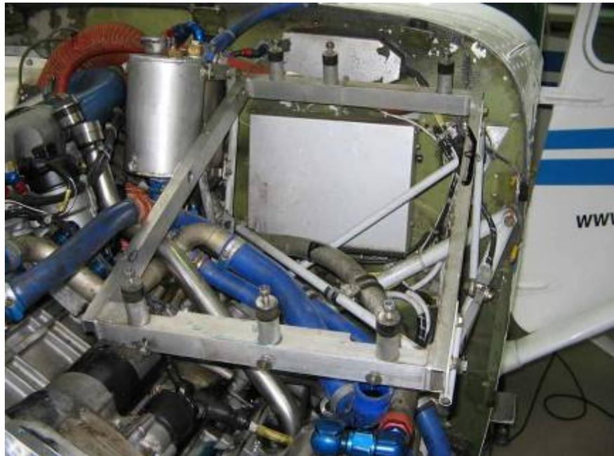
Figure 1 Oil and Water Cooler Mount
