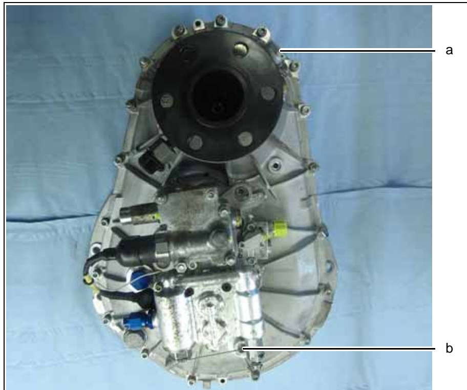
Fig. 6.25 Gearbox oil filler screw and inspection glass
