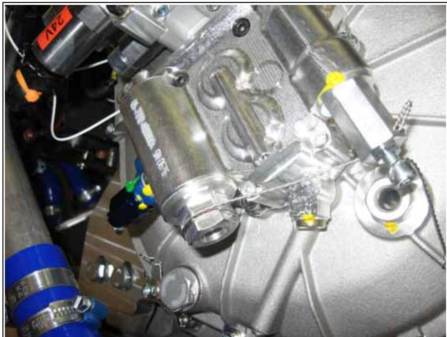
Fig. 6.20 Lock wiring the oil filter cap, the proportional pressure reducing valve and the gearbox housing
