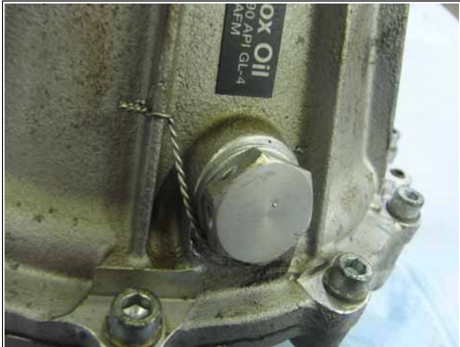
Fig. 6.48 Lock wiring the oil filler screw
