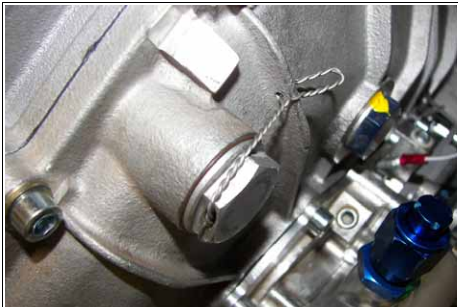
Fig. 6.54 Lock wiring the oil drain screw
