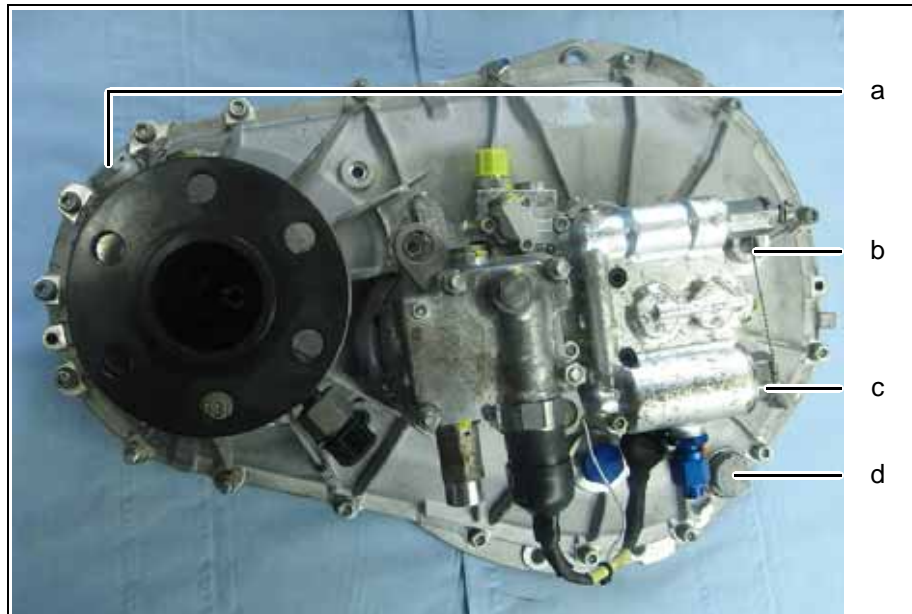
Fig. 6.49 Overview of the gearbox inspection points
