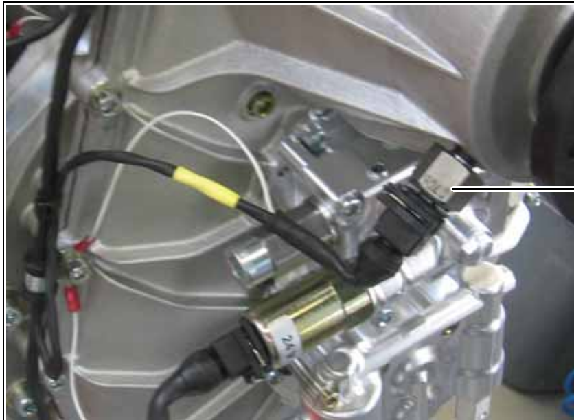
Fig. 6.10 Gearbox temperature sensor a Gearbox temperature sensor
