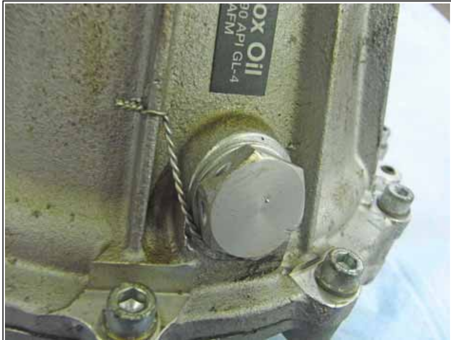
Fig. 6.26 Lock wiring the oil filler screw
