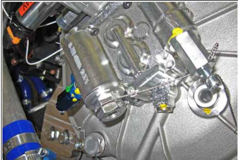
Fig. 6.53 Lock wire between oil filter cap, proportional pressure reducing valve and the gearbox housing
