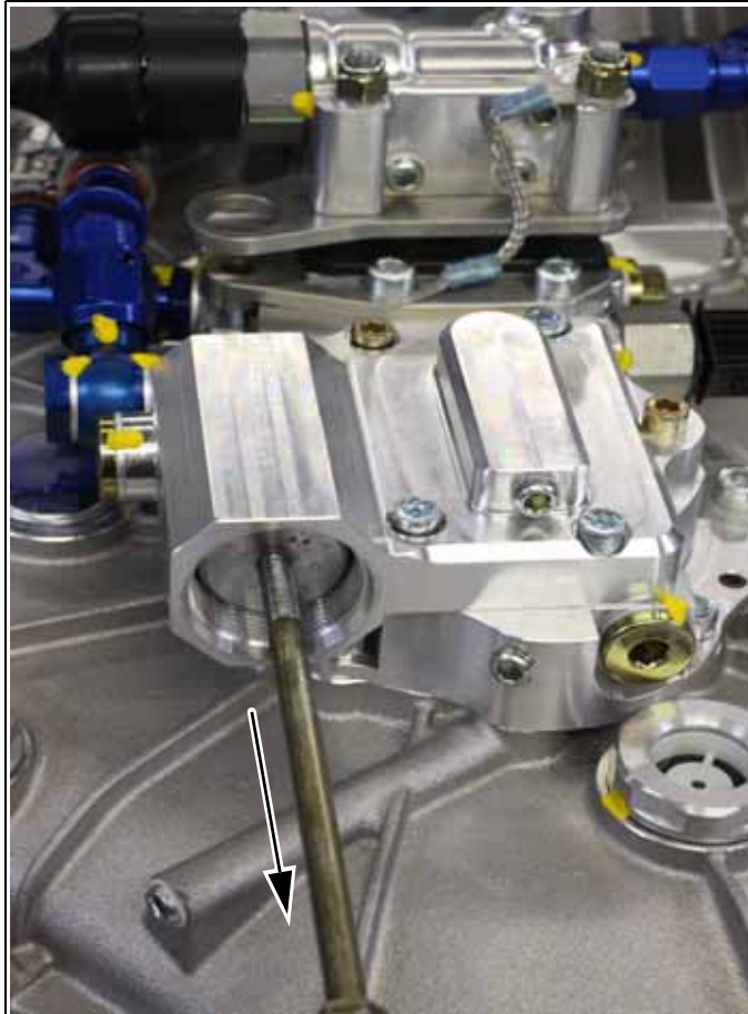
Fig. 6.44 Removal of gearbox oil filter
