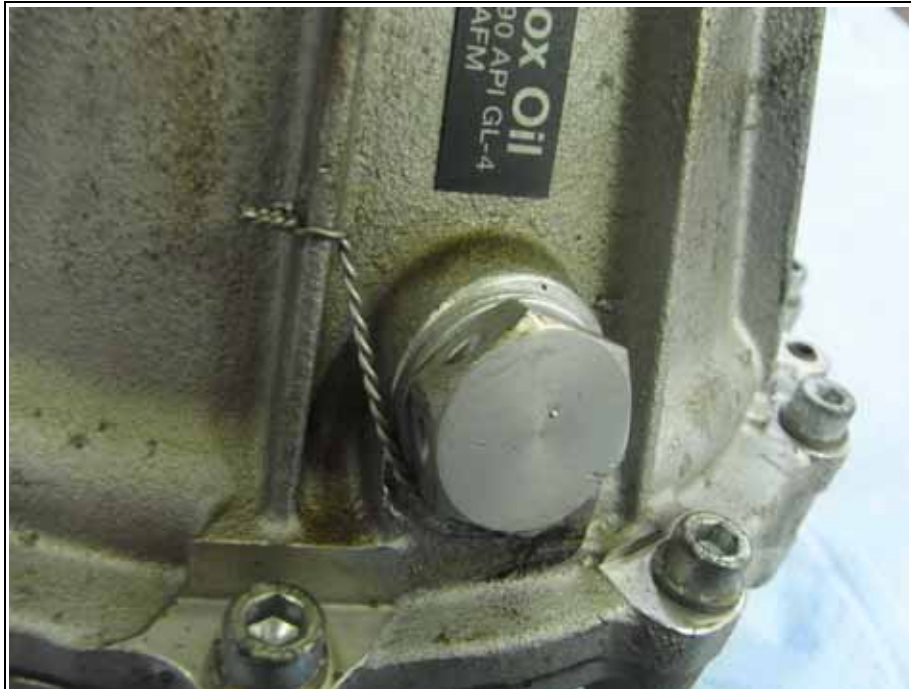
Fig. 6.55 Lock wiring the oil filler screw
