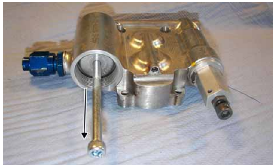
Fig. 6.17 Removal of gearbox oil filter
