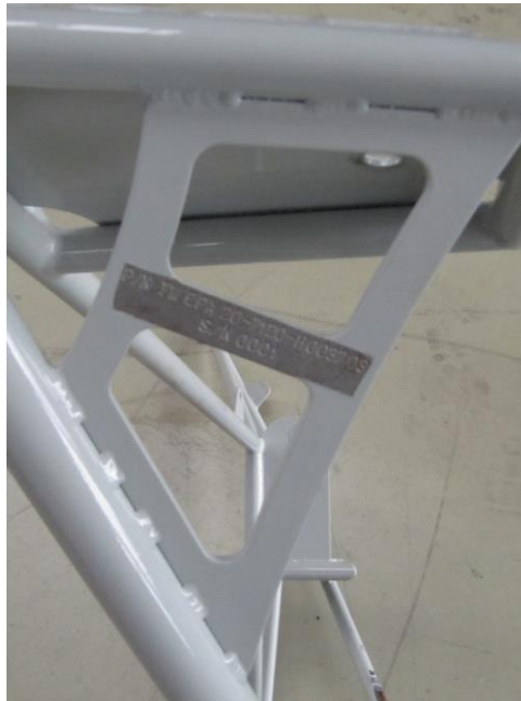
Figure 5: Welding seams & bracket to inspect
