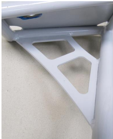
Figure 3: Missing welding seams
