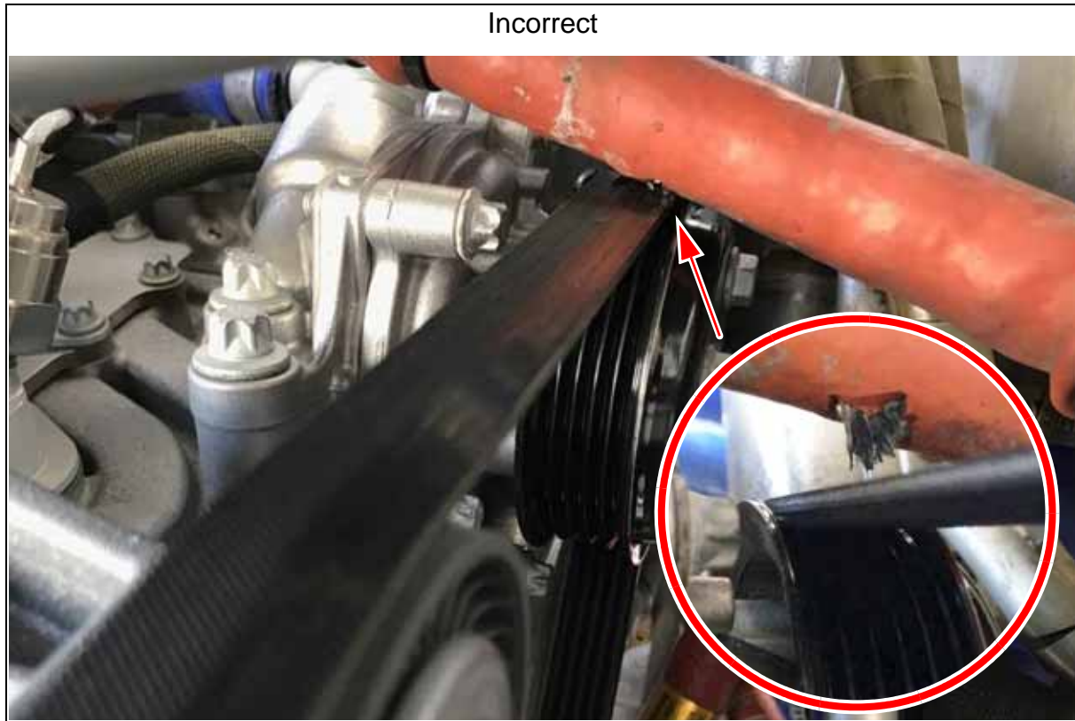
Figure 8 grindings by other parts, Check the correct mounting of other components Figure shows Diamond DA40
