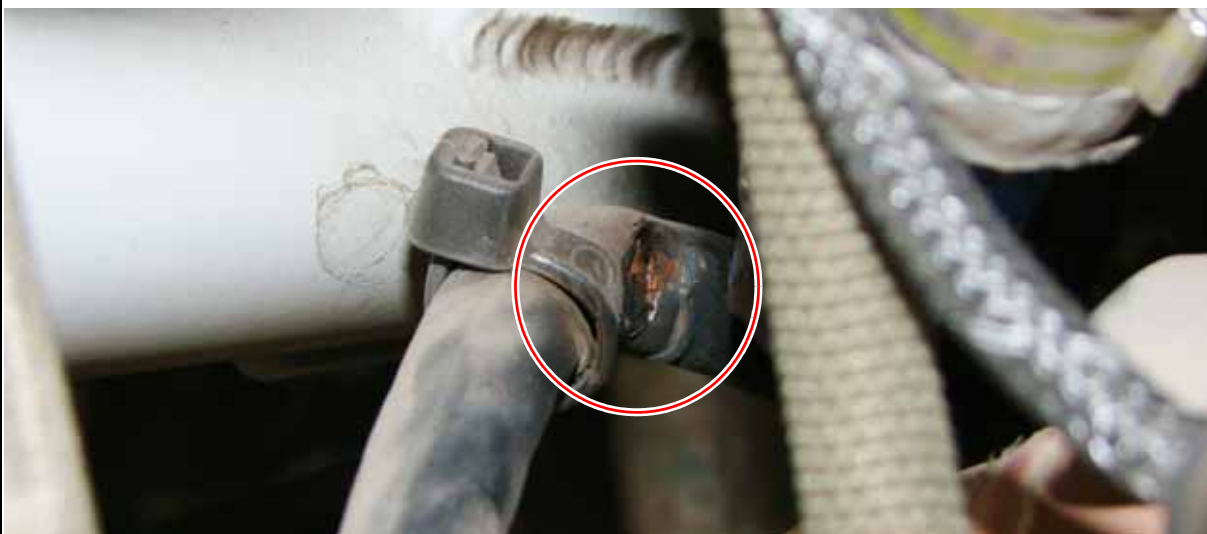
Figure 2 chafing spot: ground cable at engine mount rear right
