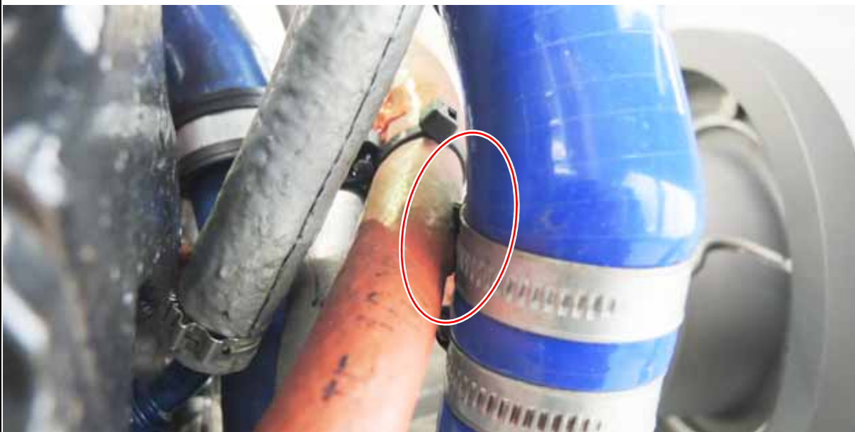
Figure 12 chafing spot: hose clamp water hose
