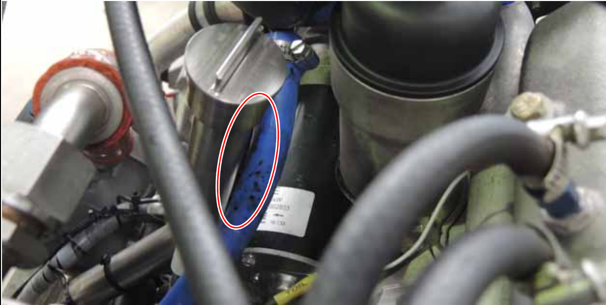
Figure 11 chafing spot: oil tube - missing cable ties
