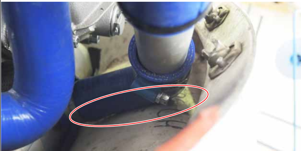
Figure 8 chafing spot: cowling DA42
