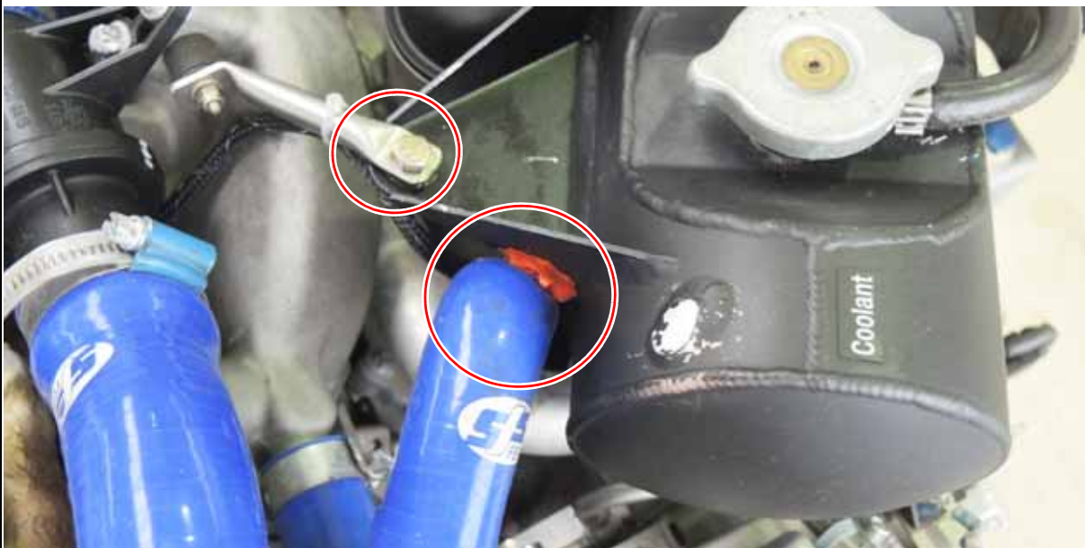
Figure 10 chafing spot: coolant tank DA42, chafing due to incorrect installed bracket
