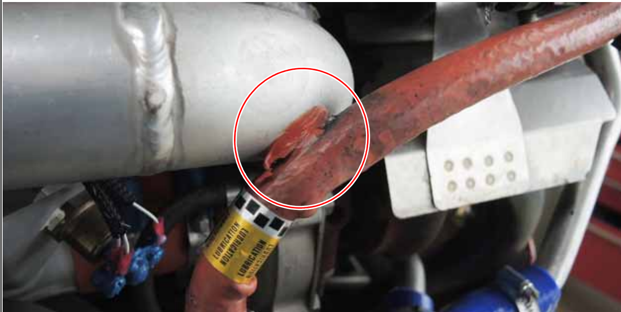
Figure 13 chafing spot: turbo pipe
