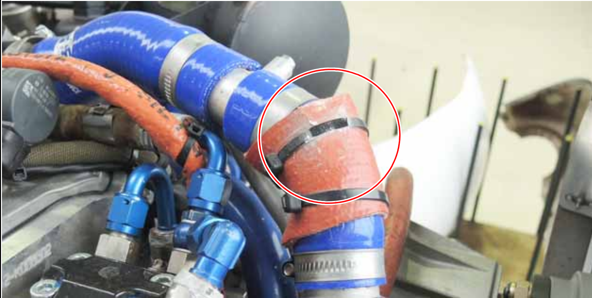
Figure 9 chafing spot: cowling DA42
