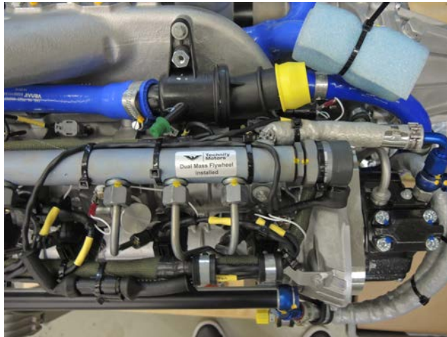
Fig. 1 – Label Dual Mass Flywheel
