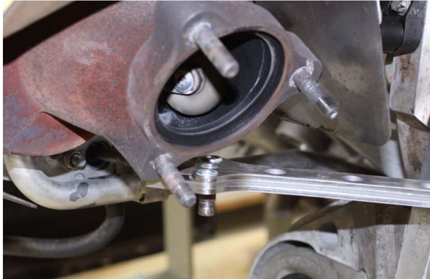
Fig. 2 Hold the waste gate lever steady
