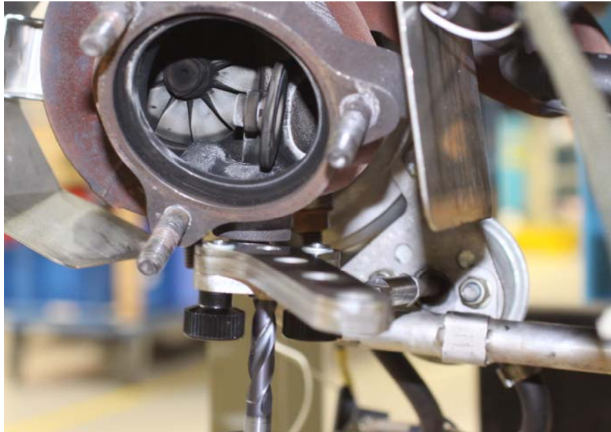
Fig. 5 Drilling the hole for the new pin
