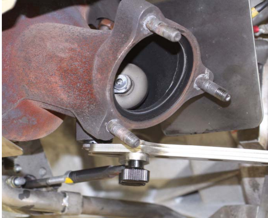
Fig. 4 Installation of the drill guiding tool
