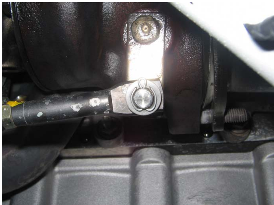
Fig. 7 Attachment of the adjustment endpiece on the waste gate lever
