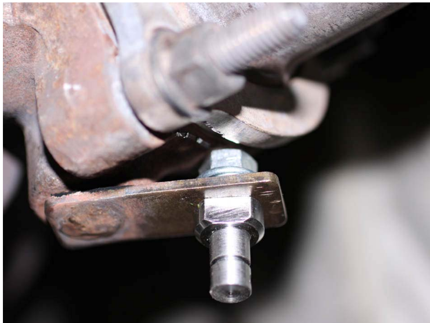
Fig. 6 Attachment of the new pin
